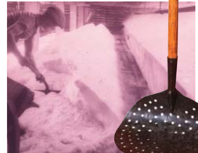
Right: Skimmer used to sift salt out of pans. Below: Open pan salt production.
